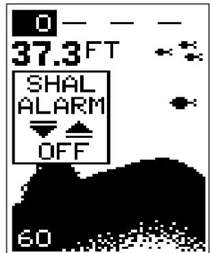
alarm setting. When the number reaches the desired setting, release the arrow key. When the bottom depth goes shallower than the alarm's setting an alarm tone sounds. At the same time the alarm sounds, a message box appears on the screen as shown at right.
