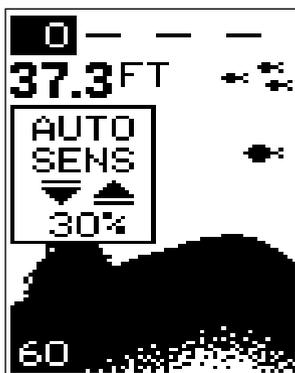
After you've adjusted the unit to the desired sensitivity level, press the ON/CLEAR key to clear the display; or wait a few seconds and it will automatically clear.
