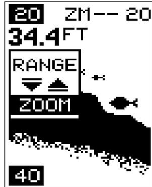
To turn the zoom feature off, press the menu key until the RANGE/ZOOM menu appears. Now press the up arrow key. This switches the unit into the range mode, which turns the zoom feature off.
