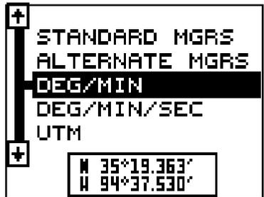
The Eagle View can show the position in degrees, minutes, and thousandths of a minute (36 28.700') or degrees, minutes, seconds, and tenths of a second (36 28' 40.9"). It can also show position in UTM's (Universal Transverse Mercator) projection, British, Irish, and Military Grid systems.
