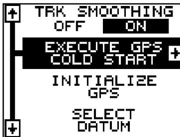
To view these menu items, press the MENU key, then highlight the “GPS Setup” menu. Press the right arrow key. The screen shown above appears.
