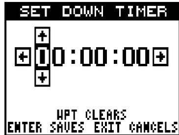
Using the right and left arrow keys, move the black box to the first number in the time that you want to set. (The time is in hours, minutes, and seconds) Now press the up or down arrow keys until the desired number shows. Continue until the time shown in the display is correct, then press the ENT key.
