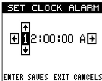
To turn the alarm on, press the MENU key, then highlight the "CLK ALM" menu. Press the right arrow key. The alarm is now activated.
