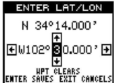
Keep pressing the arrow keys until the latitude and longitude are set to your local position. (Note: This position does not have to be very accurate. If you can get it within one degree of your actual position, that will be fine.) When it's set, press the ENT key. The Eagle View accepts your entry and returns to the GPS setup menu.
