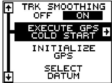
The unit will begin searching for the satellites. It can take as long as 5 minutes for it to lock on to the necessary satellites. Remember, when it does, your local time and possibly date can be wrong. Use the method shown in the initialization section at the front of this manual to change them, if needed. Once this is done, an internal clock will keep the correct time, even when the unit is turned off. The GPS system updates this clock when the unit is locked on to the satellites.
