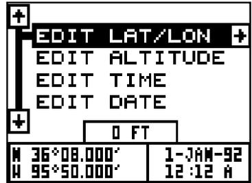
To change the position, press the right arrow key while the "EDIT LAT/LON" box is highlighted. The screen shown at right appears.
