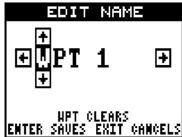
Press the up or down arrow keys to select the first letter in the name. Press the right arrow key to move the black box to the next position in the name. Repeat this sequence until you've entered all of the letters in the waypoint name. Press the ENT key to accept this name, the WPT key to erase all characters in the name, or the EXIT key to leave this screen without saving any changes.
