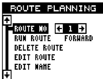
This unit can store up to twenty different routes. Route number one shows on this page. If you wish to create a route using a different number, simply press the left or right arrow keys until the desired route number appears. In this example, however, we'll use route number one.
