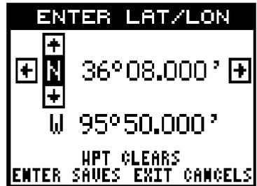
If your latitude is south, press the up or down arrow key to change it. If it is north, press the right arrow key to move the change box to the first number in the latitude. Now press the up arrow key to increase the number or the down arrow key to decrease it. Once the first number in the latitude is set, press the right arrow key once to move to the next number in the latitude.
