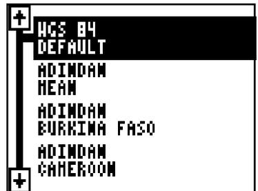
The WGS-84 label is highlighted. To change it, simply press the up or down arrow keys to highlight the desired datum, then press the ENT key. This selects the datum and erases the select datum menu.
