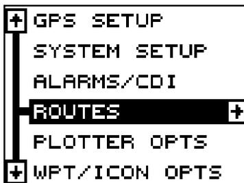
Using the arrow keys moves the black box to highlight different menus on the list. Pressing the right arrow key selects the menu.
