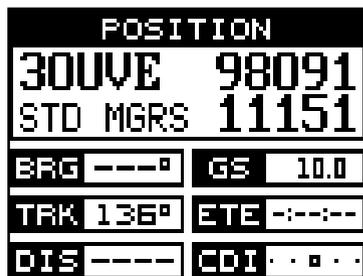
Press the up or down arrow keys to highlight the desired position format. Press the EXIT key to both select the format and erase the position format menu.
