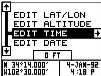
Once the Eagle View finds and locks on to three satellites, it stops flashing the numbers on the display. (Note: Altitude will still flash until the unit locks on to the fourth satellite. It takes four satellites to determine altitude.)
