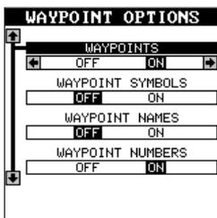
You can turn all of the user waypoints on or off (Waypoints), an icon (Waypoint Symbols), its name (Waypoint Names), or its number (Waypoint Numbers). Press the up or down arrow keys to move the black box to the desired menu, then press the right arrow key to turn it on. Press the EXIT key to erase this menu.
