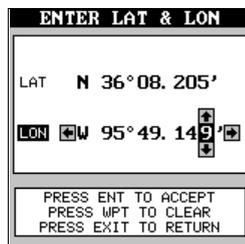
When you're ready to save this position and return to the waypoint screen, press the ENT key. The location you entered shows at the bottom of the screen under the waypoint number you selected.
