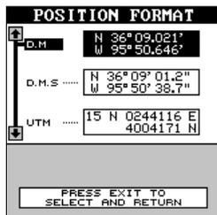
Press the up or down arrow keys to highlight the desired position format. Press the EXIT key to select the format and erase the menu.
