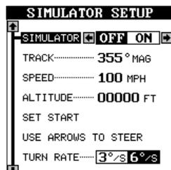
To change either the track or speed, highlight the one you want to change, then press the right arrow key. Use the up and down arrow keys to change each number, then use the left and right arrow keys to select the other numbers that you wish to change.
