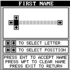
This is the first name entry screen. Press the up or down arrow keys until the first letter appears that you want to use. When it does, then press the right arrow key to move to the next letter. Continue this process until the I.D. is complete. You can press the WPT key to completely erase all of the characters you entered and start over, if you need to. Pressing the EXIT key erases this screen without accepting any input. When the first name is correct, press the ENT key.
