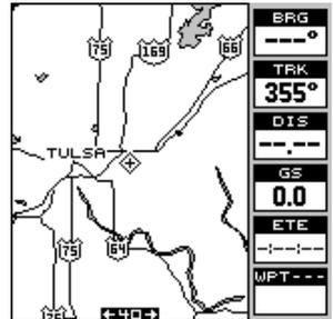
This is Map 3. Your present position is shown as a cross surrounded by a diamond. As you wait for the AccuMap 12 to find your position, you'll see numbers flashing on the display. Anytime you see flashing numbers, it means the AccuMap 12 does not have a position! Do not rely on any data that is flashing! When the numbers stop flashing, the unit has locked on to the satellites and the position is good.
