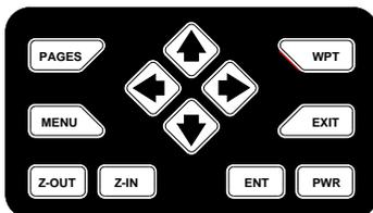
The WPT key lets you create, save, and recall waypoints and routes. The PAGES key switches the unit between the three major displays: windows, navigation, and mapping. To select different features, or to modify functions, press the MENU key. The Z-OUT and Z-IN keys zoom-out and zoom-in your view on the mapping screen. The ENT and EXIT keys let you enter or erase selections. The PWR key turns both the AccuMap 12 and its lights on and off.
