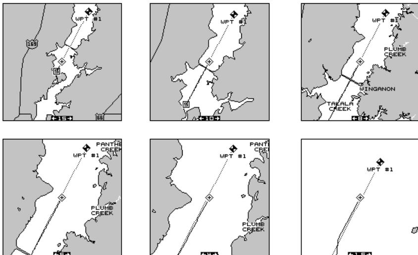
To use the autozoom feature, first set the AccuMap 12 up to navigate to a waypoint. (See the Navigation section for more details.) Next, simply press the MENU key, then use the up or down arrow keys to highlight the “AUTOZOOM OFF/ON” menu. Press the right arrow key to turn it on, the left to turn it off.
