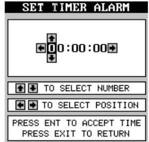
You can reset either alarm to the time you originally set by pressing the MENU key, then moving the black box to either the “Up Timer Reset” or “DN Timer Reset” label, then press the right arrow key.
