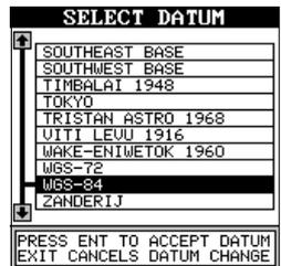
The WGS-84 label is highlighted. To change it, simply press the up or down arrow keys until the desired datum is highlighted, then press the ENT key. This selects the datum and erases the datum menu. The AccuMap 12 is now using the datum you selected.
