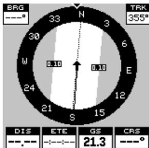
Your speed over ground or Ground Speed is shown at the bottom of this screen. In this example, the ground speed is 21.3 miles per hour. The screen looks like this when you're not navigating to a waypoint. (See page 39 for information on waypoint navigation.) If you navigate to a waypoint, the screen looks like the one below.
