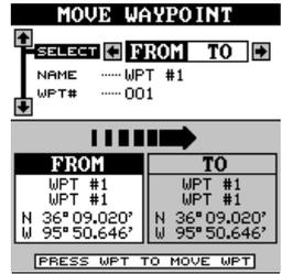
Once you have the desired waypoint showing on the screen that you’re going to be moving the information FROM, then you need to choose the waypoint number that you’re going to move that information TO. Highlight the “Select” label at the top of the screen, then press the right arrow key to select “TO”. Now choose the waypoint number that you wish to move the information to. In this example, we selected waypoint number 10.
