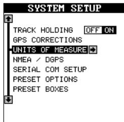
To change a unit of measure, first select the "Units of Measure" from the "System Setup" menu. The screen shown at right appears. To change a setting on this menu, highlight the desired selection, then press the left or right arrow key. You can change one or all of the settings on this page. When you're finished, press the EXIT key.
