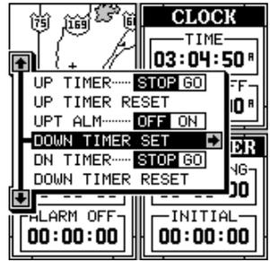
To start the timer, press the MENU key, then move the black box to the “Dn Timer STOP/GO” label. Press the right arrow key to start the timer. The timer continues counting until you stop it. If you turn the up timer’s alarm on (press the right arrow key when the black box is on the (Up ALM...Off/On label), it will sound a tone when it reaches the time you entered in the up timer set menu. Press the EXIT key to silence the alarm.
