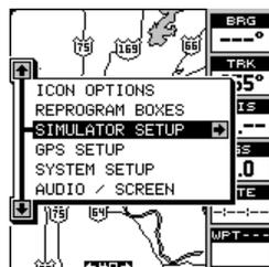
If you simply press the right arrow key, turning the simulator on, the AccuMap 12 will start from your present position and follow a track of 355° at 100 miles per hour.
