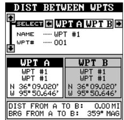
“Select WPT A” label is highlighted. Now press the down arrow key to highlight either the name or waypoint number labels. You can select a waypoint by name or number. In this example, we used the number method and we’re going to measure the distance between waypoint numbers three and four.
