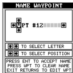
Press the up or down arrow keys to select the first letter in the name. Press the right arrow key to move the black box to the next position in the name. Repeat this sequence until you've entered all of the letters in the waypoint name. Press the ENT key to accept this name, the WPT key to erase all characters in the name, or the EXIT key to leave this screen without saving any changes.
