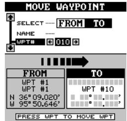
When everything on this screen is correct, press the WPT key. In this example, the name, icon, and position were moved from waypoint number 1 to waypoint number 10. Press the EXIT key to erase this screen when you’re finished.
