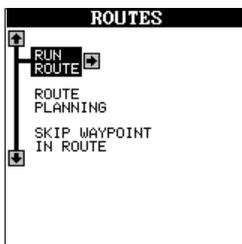
To create a route, first press the MENU key, highlight the "ROUTES" label, and press the right arrow key. The screen shown above appears. Next, highlight the "ROUTE PLANNING" label and press the right arrow key. The route planning screen shown at right appears.
