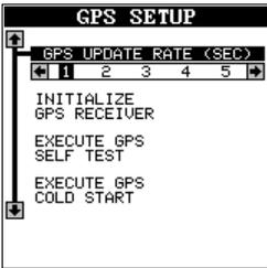
To view these menu items, press the MENU key, then highlight the “GPS Setup” menu. Press the right arrow key. The screen shown at right appears.
