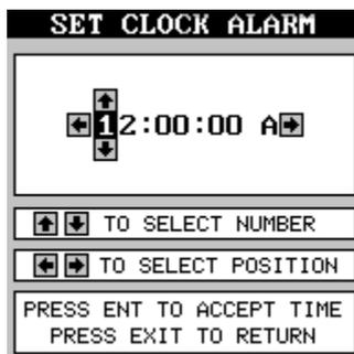
To turn the alarm on, press the MENU key, then select the “CLK ALM” menu. Press the right arrow key. The alarm is now activated.
