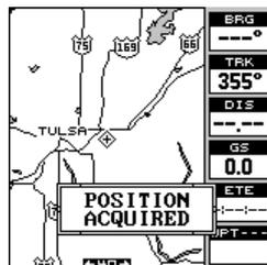
To turn on either message, select the "GPS Alarms" menu from the main menu, then move the black box to the desired message and press the right arrow key to turn it on. Press the EXIT key to erase this screen.
