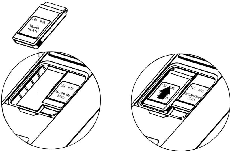
To install a cartridge into the AccuMap 12, *first make certain the unit is turned off. Never install or remove a cartridge with the unit turned on!* You can damage your unit if you install or remove a cartridge with the unit turned on. Next, pry the cover off the back of the unit. Place the cartridge into either slot with its label facing you as shown at the bottom of the previous page. Now slide the cartridge towards the top until it stops. Replace the cover.
