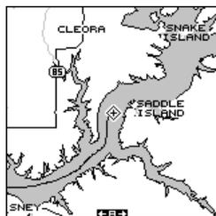
Use the Z-OUT and Z-IN keys to enlarge or reduce the mapping area. If you have an IMS SmartMap™ cartridge installed, it's detail typically begins showing when you zoom in to the 10 mile range.
