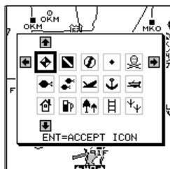
Press the arrow keys to highlight the desired icon, then press the ENT key to assign it to your waypoint. The unit returns to the waypoint screen with the icon you selected assigned to the waypoint.
