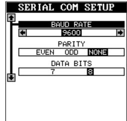
Check your DGPS receiver's manual for the proper data settings. Highlight the menu item you need to change. Press the left or right arrow keys to change them. The serial port defaults are 4800 baud, no parity, and 8 data bits. Press the EXIT key to erase this menu.
