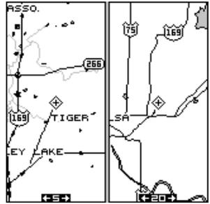
When you press the MENU, ZOOM IN or OUT, or ENT keys, a message appears asking you which display you want to affect. On the screen shown at right, the menu key was pressed. The unit wants to know which map you want to change. Press the left arrow key for the left map, the right arrow key for the right map. The main menu then appears.
