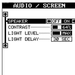
The backlights brightness is also adjustable. To do this, highlight the "Light" menu. Now press the left or right arrow key until you have the lights at the desired level. Press the EXIT key when you're finished. The default light level is maximum.
