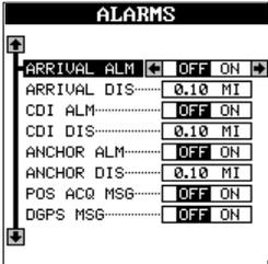
To adjust the alarm's distance, move the black box to the alarm's "DIS" menu item, then press the right or left arrow keys to increase or decrease the alarm's distance.
