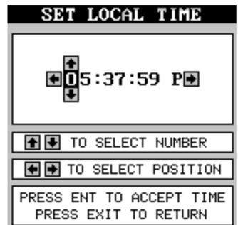
Using the right and left arrow keys, highlight the first number in the time that you want to change. Now press the up or down arrow keys until the desired number shows. Continue until the time shown in the display
