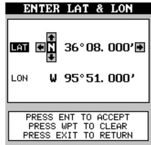
Keep pressing the arrow keys until the latitude and longitude are set to your local position. (Note: This position does not have to be very accurate. If you can get it within one degree of your actual position, that will be fine.) When it's set, press the ENT key. The AccuMap 12 accepts your entry and returns to the GPS setup menu.
