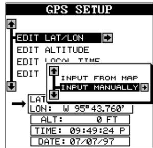
If your latitude is south, press the up or down arrow key to change it. If it is north, press the right arrow key to highlight the first number in the latitude. Now press the up arrow key to increase the number or the down arrow key to decrease it. Once the first number in the latitude is set, press the right arrow key once to move to the next number in the latitude.
