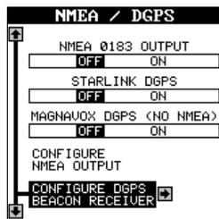
These menus select the beacon receiver’s frequency and bit rate (in bits per second). If you are using a Starlink receiver, turning the auto mode on causes the AccuMap 12 to auto-detect the frequency and bit rate.
