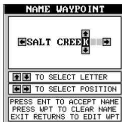
Tip: You can select waypoints by name instead of by number. Simply press the right arrow key while the black box is on the "Name" portion of the waypoint menu, then press the up or down arrow keys until the desired waypoint name appears.
