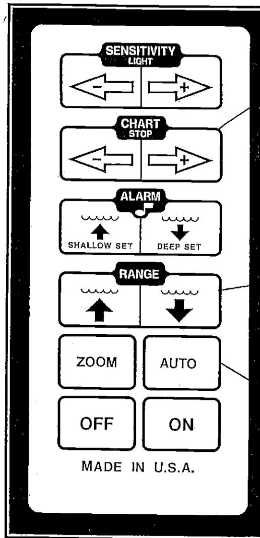
**CHART** The chart speed is controlled by the CHART group of keys. The Z-6100 has 32 chart speeds, ranging from very slow to FAST. Pressing the FAST key speeds up the chart speed. The slow key reduces it. The chart display can be stopped and started again by pressing both arrow keys at the same time.
