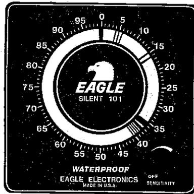
Small minnows or bait fish appear on the dial as thin, pale lines. If they are tightly schooled they may cover a depth of from five to ten feet on the dial with a few pale lines for individual minnows at the bottom of the school. Your EAGLE will indicate even a single minnow 30 feet beneath the surface of the water.
