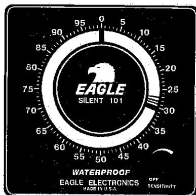
When you are hunting fish, with the gain adjusted properly to return a clear, bright signal from a bottom of gravel, sand, or shell, you will sometimes see the signal disappear. This doesn't mean that you have suddenly come to extremely deep water — the dial would have shown the drop-off with a wide band of signals in this case.
